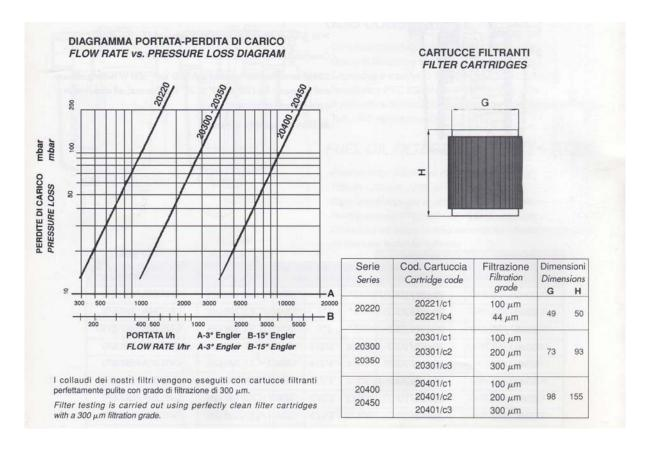
Filter testing is carried out using perfectly clean filter cartridges with a 300  $\mu m$  filtration grade.
